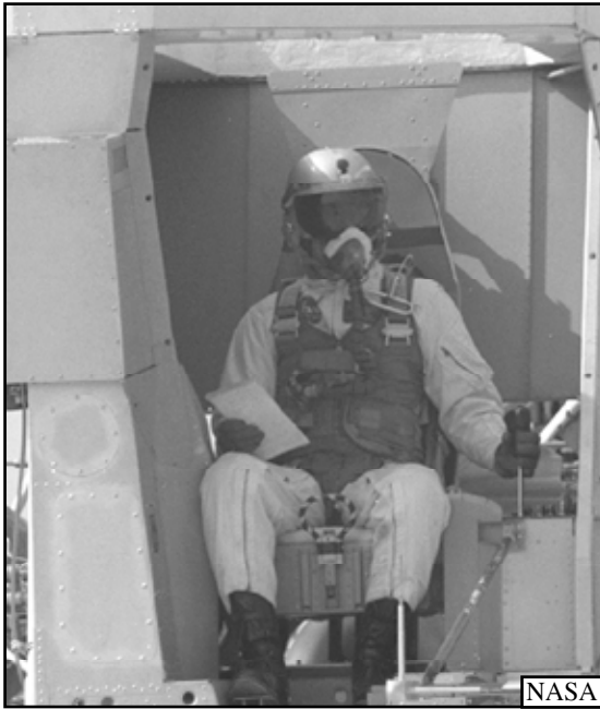
25 October 1969, Astronaut Charles Conrad Jr., sits in the cockpit of a Lunar Landing Training Vehicle during a training exercise designed to help the mission commander practice lunar landing techniques with the Lunar Module.
