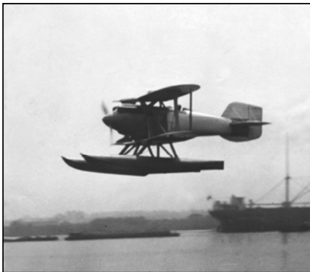
Wright RW-2 racing seaplane piloted by LT A. W. Gorton in 1925. Its speed averaged 173 miles per hour
